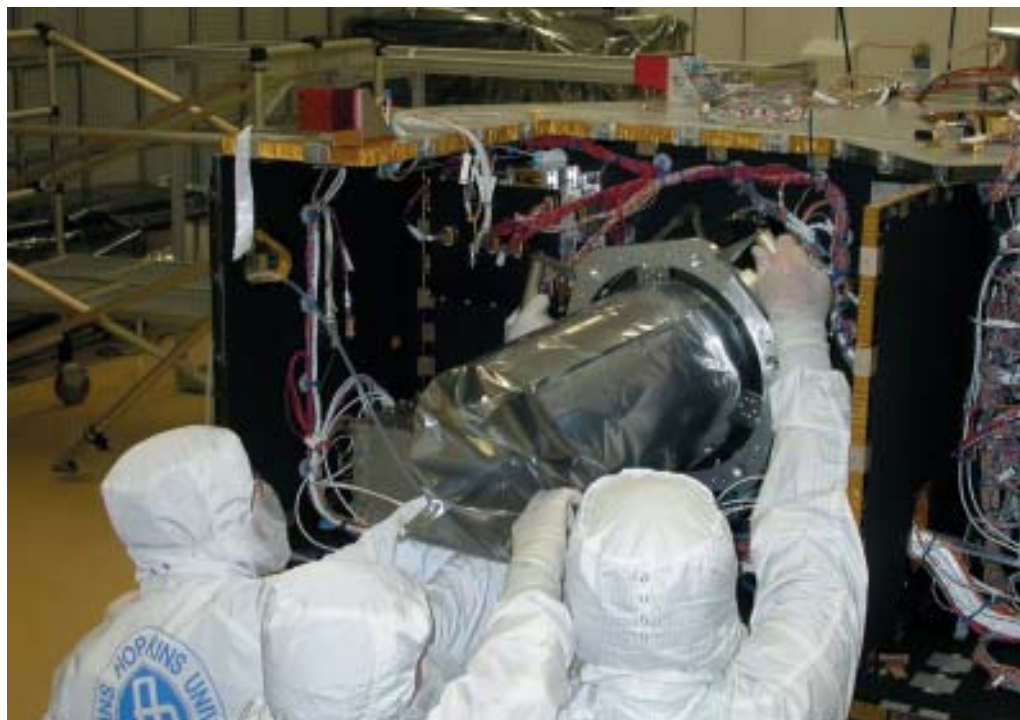
Technicians install the Long Range Reconnaissance Imager (LORRI) on New Horizons spacecraft. The telescopic camera is one of seven science instruments designed for the Pluto flyby mission. JHUAPL/SwRI
